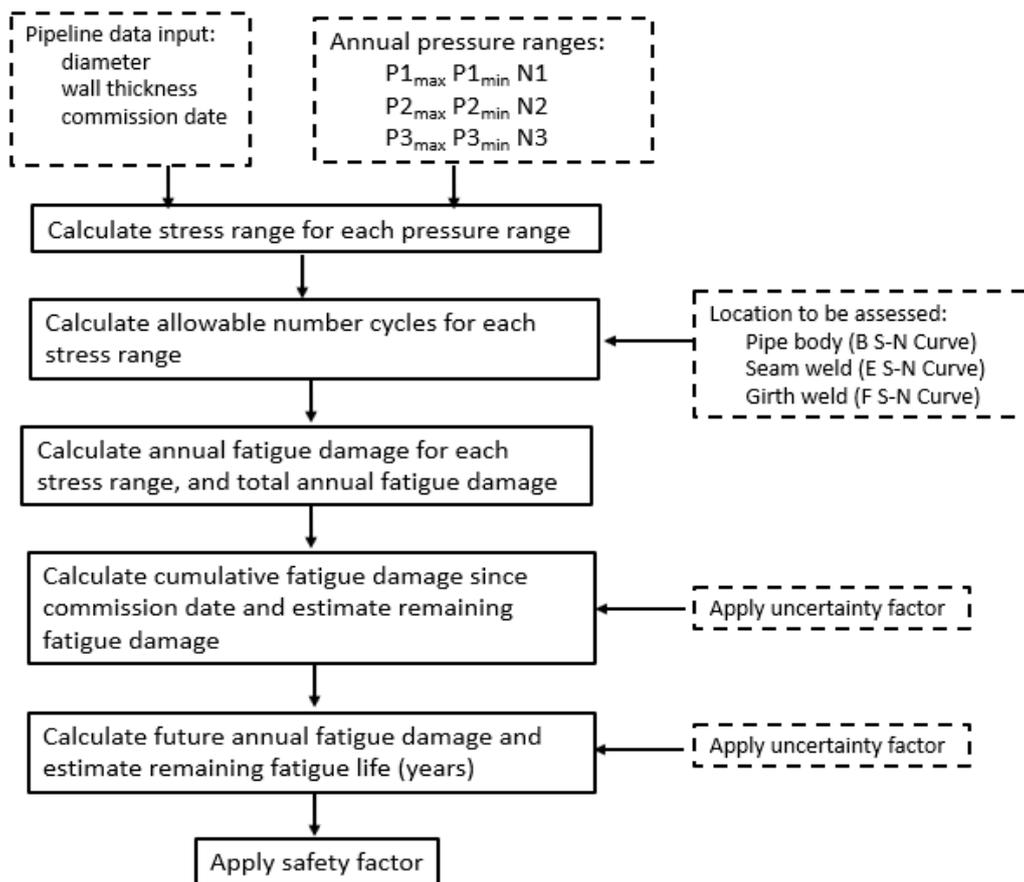
**Figure A2.1 Fatigue Calculation Methodology**
