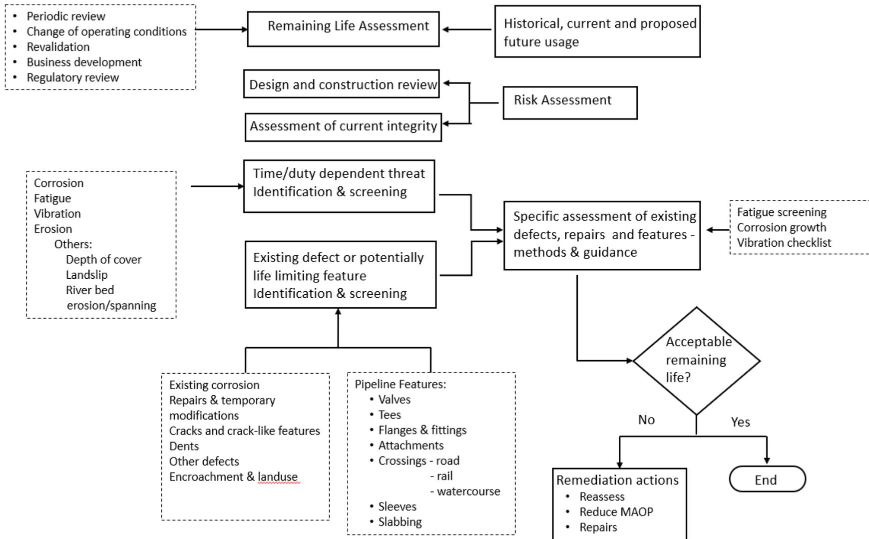
**Figure 2 Process for Assessment of Remaining Life**
