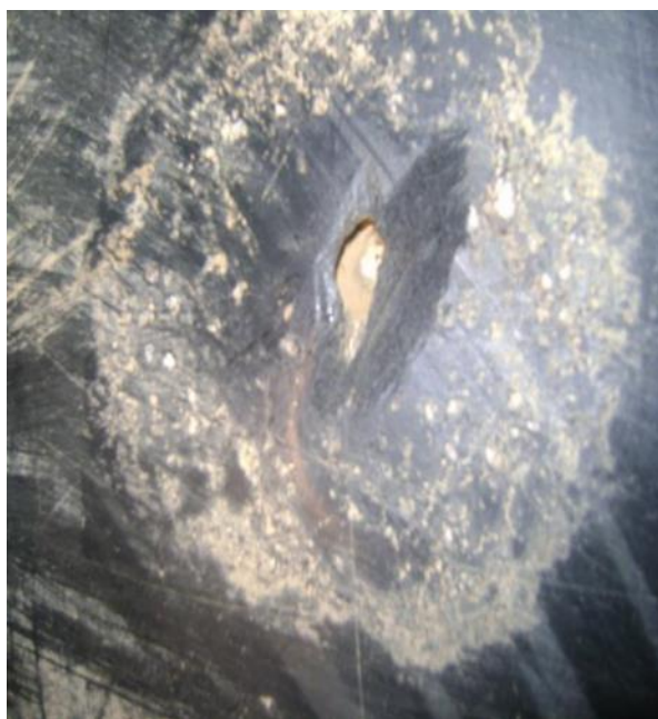
Figure 10 Picture of lightning damage to a buried pipeline. The damaged resulted in through wall penetration on a high-pressure gas pipeline.
