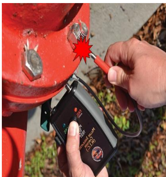
Figure 14 Spark risk on testing I/F with high frequency insulation flange tester with a.c. voltage present
