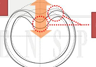
cyclic internal pressure induces cyclic stresses and strains in the dent
