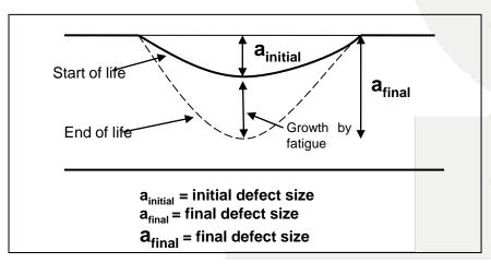
Calculating the largest crack type defect that would have survived the pipeline's precommissioning hydrotest;
