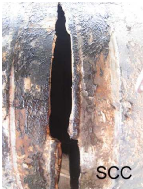
Figure 7: Circumferential SCC failure
