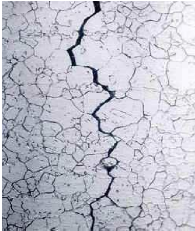
Figure 3: Intergranular crack growth
