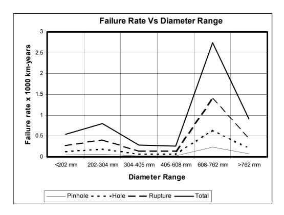
This is an unusual trend for pipeline failures – normally larger diameter pipelines show lower failure rates than smaller diameter pipelines. Also, pipeline rupture is the smallest contribution to failure rates, whereas in the Atkins analysis, it appears to be the largest contribution.
