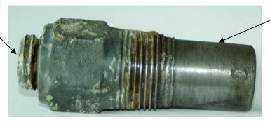
stem sealing compound injector body (hexagonal casing)
