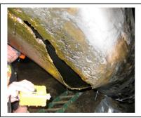
There was no evidence of a pressure excursion or upset conditions prior to the failure. Pressure at the leak location was 694 psig at time of the failure (established Maximum Operating Pressure of this segment is 1050 psig). There were no injuries and no impact to wildlife as a result of the release or follow-up response activities.
