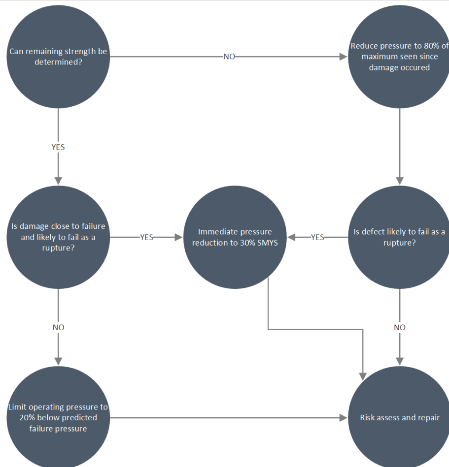
Figure 6-3: Pressure reduction guidance following detection of anomaly
