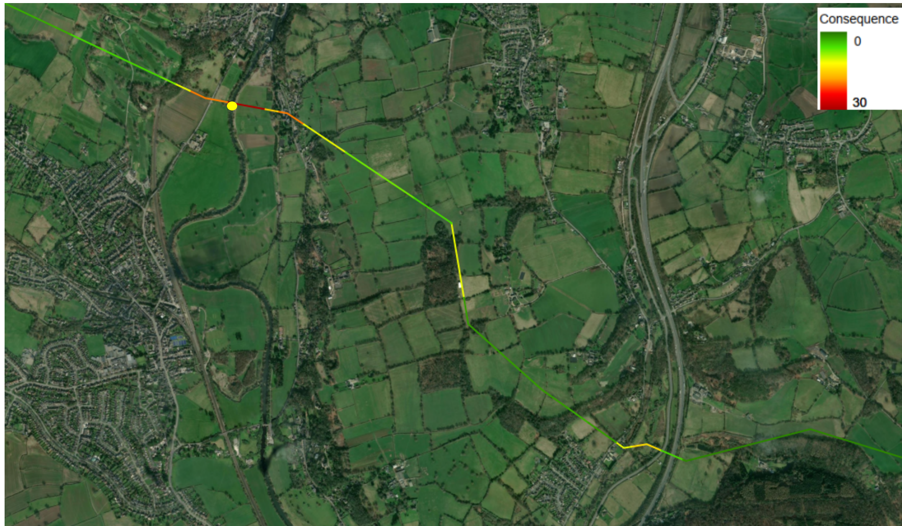
Figure 5.2 – Example Pipeline Consequence Output
