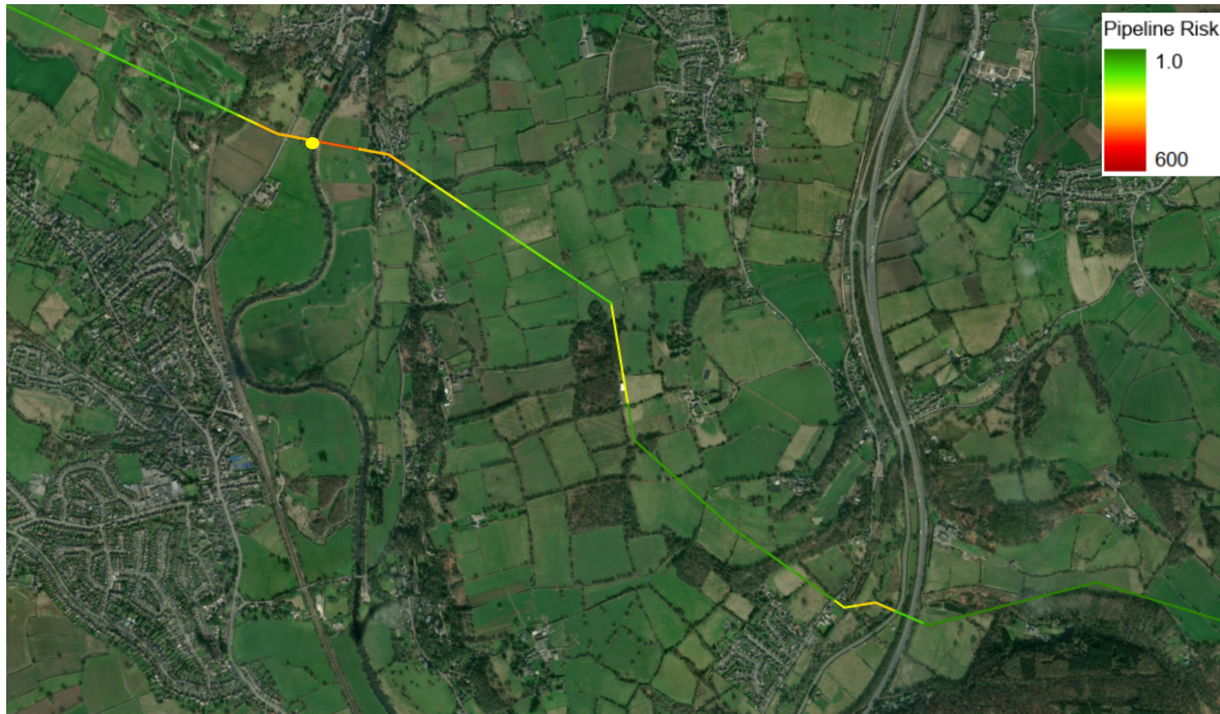
Figure 6.1 – Example Pipeline Risk Output
